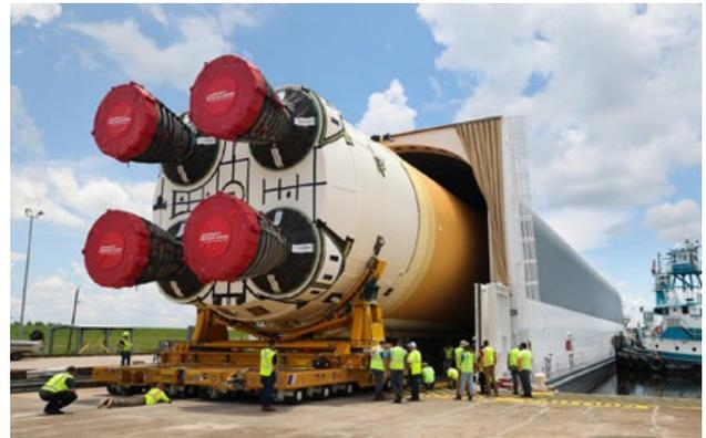
The Artemis 2 Space Launch System core stage being loaded into the Pegasus barge at Michoud Assembly Facility, July 16, 2024. © NASA Michoud Assembly Facility / NASA/Steven Seipel
