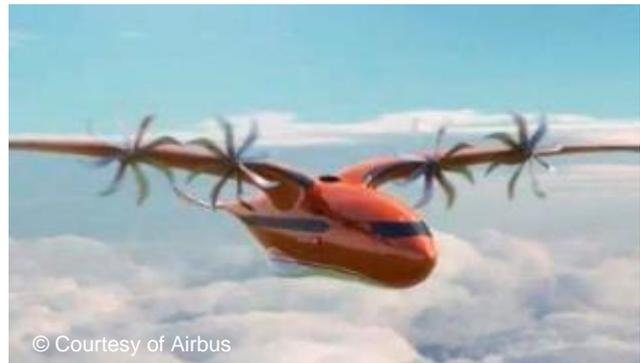
The final demonstration is a regional aircraft with technologies ready for entry into service by 2035, incorporating product-viable solutions for technologies, integration, infrastructure, and certification. The aircraft will include hybrid-electric propulsion supported by 100% drop-in fuels or hydrogen whether fuel cells or H2 burning for the thermal power source, to reach up to 90% lower emissions while being fully compliant with ICAO noise rules.
