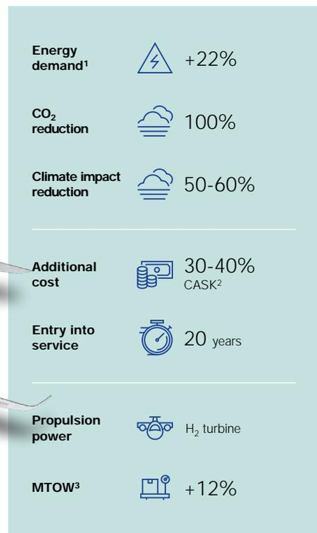
1. Major assumptions: 37% gravimetric index of LH<sub>2</sub> tank, 92% useable LH<sub>2</sub> fuel, 47% H<sub>2</sub> turbine cruise efficiency, 80% fan efficiency
