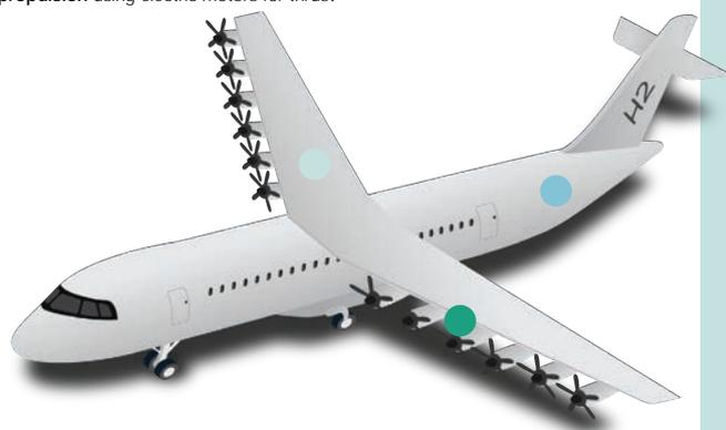
1. Major assumptions: 30% gravimetric index of LH<sub>2</sub> tank, 90% useable LH<sub>2</sub> fuel, FCS mass 1.75 kW/kg (incl. cooling) and 59% peak efficiency (LHV), e-motors and PMAD with 97%
