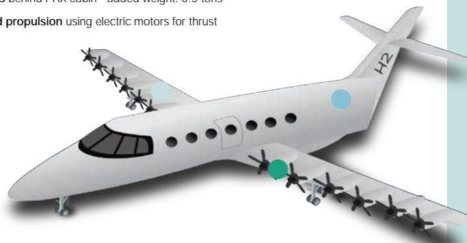
1. Major assumptions: 25% gravimetric index of LH<sub>2</sub> tank, 90% useable LH<sub>2</sub> fuel, FCS mass 1.5 kW/kg (incl. cooling) and 58% peak efficiency (LHV), e-motors and PMAD with 97% efficiency, battery with 0.6 kWh/kg
