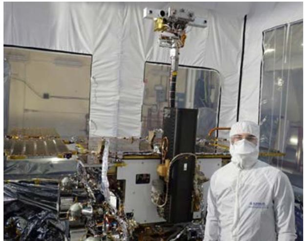
*The ExoMars - Rosalind Franklin - Rover during the environmental testing phase at Airbus Toulouse. Strict planetary protection measures have been applied throughout the project to keep biological contamination under acceptable limits. Credit: Airbus*
