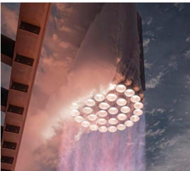
The 33 Raptor Engines of SpaceX Heavy Booster ignite during IFT-3 of Starship rocket on March 14, 2024. (Image credit: SpaceX via X)
