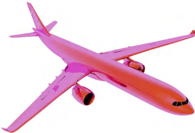
*Efficient long-range aircraft with UHBR engines and laminar flow wing.
