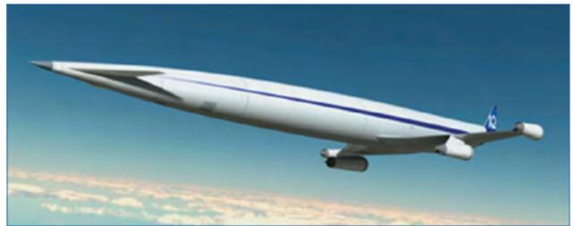
*Figure 1 – Mach 5 hydrogen based vehicle with pre-cooled turbofan-ramjet Scimitar engine. The vehicle consists of a slender fuselage with a delta wing carrying 4 engine nacelles positioned at about mid length.*
