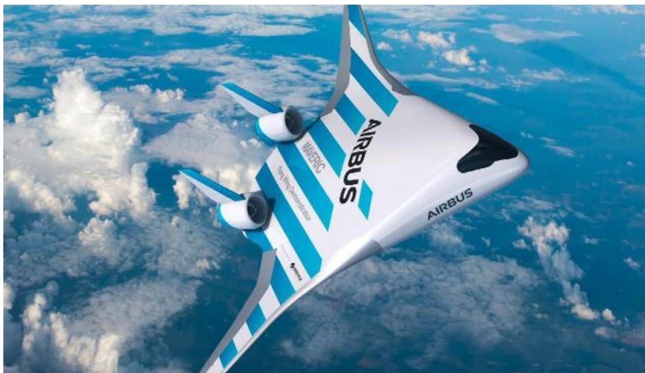
*Figure 5.1: Airbus MAVERIC Blended Wing Body concept*
